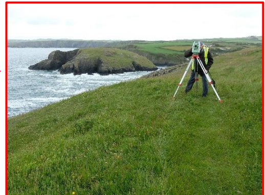
Fig. 40 Using the total station to record the wreck site.
