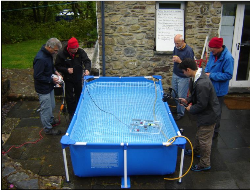
DIY ROVs under paddling pool test conditions
