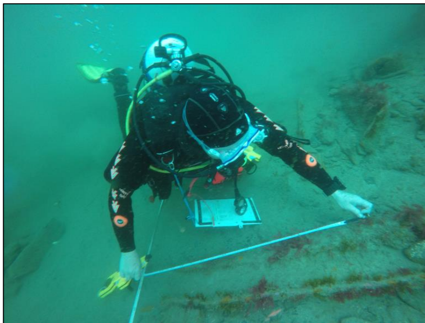
Baseline/Offset survey method in action on the SS Leysian wreck
