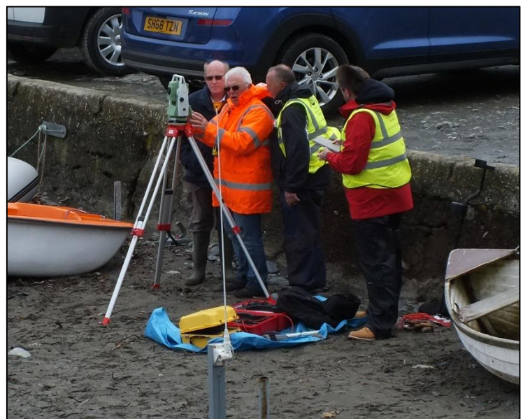
Fig. 52 Metal Detecting and recording the location of any finds using the Total Station.
