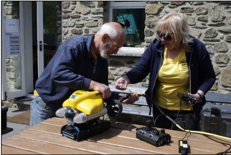
Fig. 34 The VideoRay and sonar head being assembled & tested.
